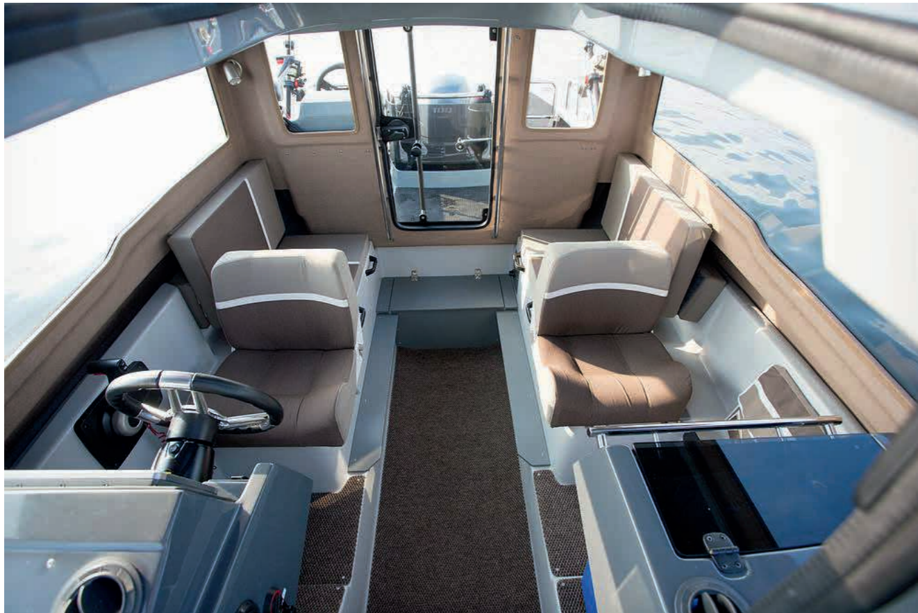
The cabin features a wide centre aisle that remains clear even when the passengers are at their seats. The large windows with narrow posts afford good visibility in all directions.
